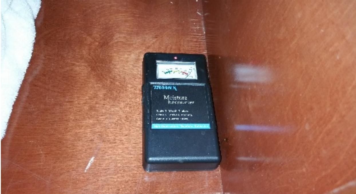
Example of kitchen cabinet having more than 20% moisture content, where trapped water is under and behind the cabinet. Cabinet box is wood veneer with particleboard. Replacement of the entire cabinet was completed.
